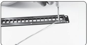
Attach one end of the grounding wire to the patch panel.
